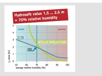
Just like the popular INTELLO airtight membrane, AEROSANA VISCONN too is humidity-variable. The sprayable sealant reacts to ambient humidity and adapts to the relevant conditions in an optimal manner. In this way, AEROSANA VISCONN and INTELLO can perform two functions: sealing to provide protection against moisture, while being extremely open to diffusion to allow for good drying out. As a result, building components are particularly well protected.
